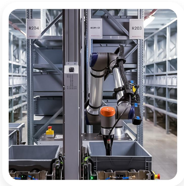
Assuming an average pick rate of 250 PPH per robotic picker and 25 PPH per AMR, a warehouse using a Goods-to-Robot system would need 4 robotic pickers and 40 AMRs to achieve a throughput of 1,000 picks per hour.
